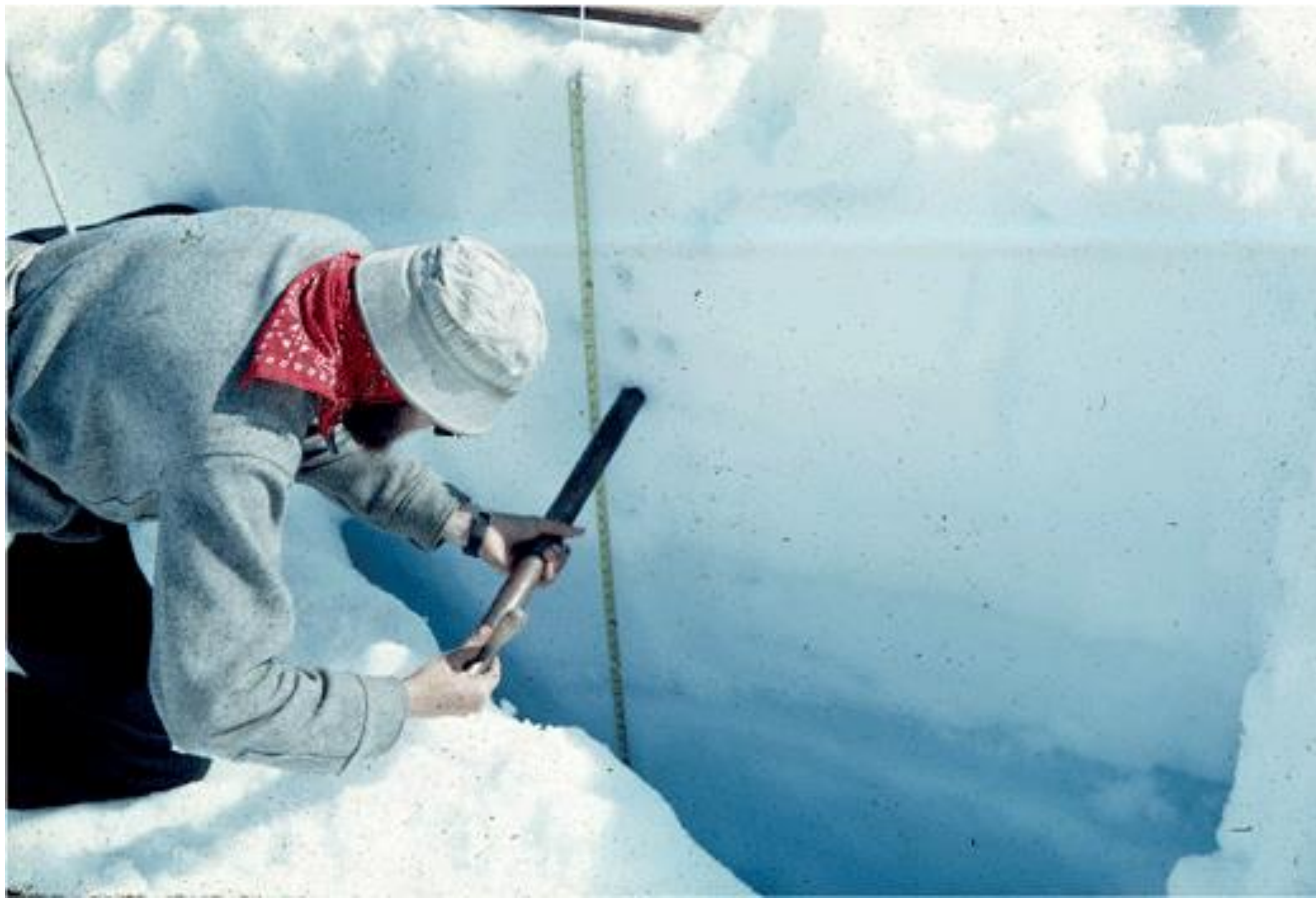
A terrestrial (!) snow pit, used for profiling snow properties (density, grain size etc.) as a function of depth
