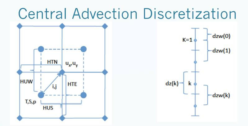
$ADV_{i,j,k} = -(u_E T_E^* - u_W T_W^*)/DXT - (v_N T_N^* - v_S T_S^*)/DYT - (w_k T_T^* - w_{k+1} T_B^*)/dz$
