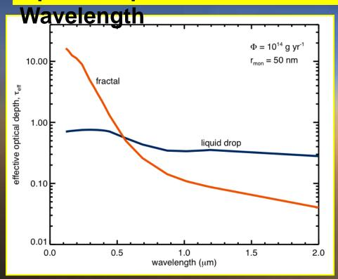
Fractal aggregates are strongly absorbing in the UV
