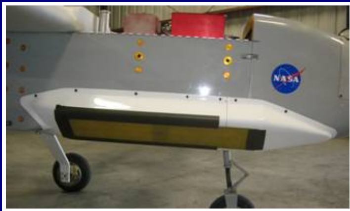
BYU mSAR panels integrated in SIERRA
