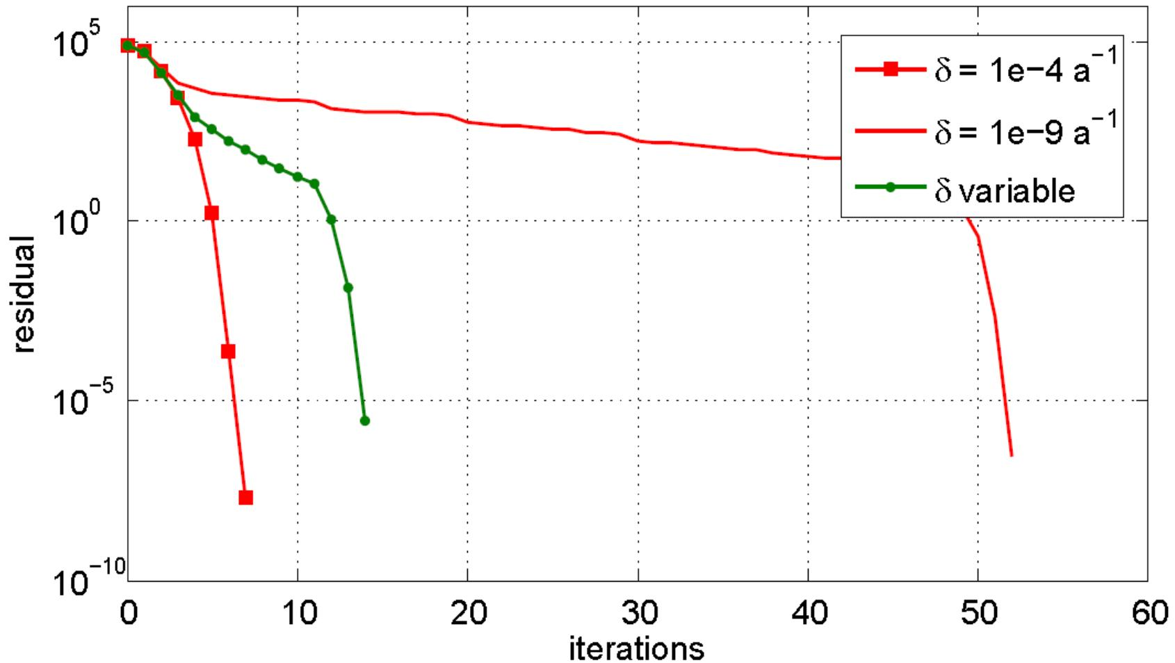
$\delta$  variable : At each newton iteration  $\delta$  is decreased from  $1e-4$  to  $1e-9$
