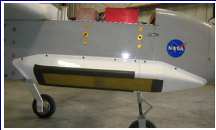
BYU mSAR panels integrated in SIERRA
