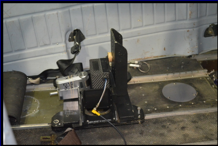
Integrated Observation System 2012 (Laser Altimeter, Video, GPS, Computer for Data Registration)
