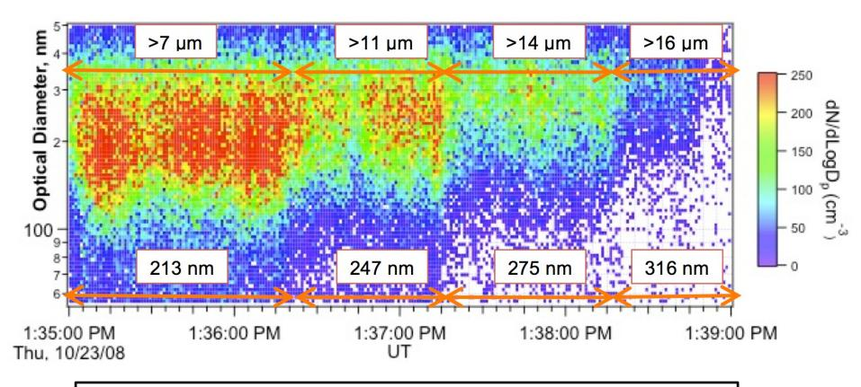
Observations taken with CVI inlet, that can selectively pass all particles above a chosen threshold size.
