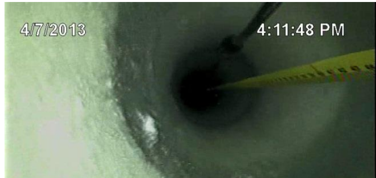
Snapshots from borehole camera taken at PFA field work site (April 2013)
