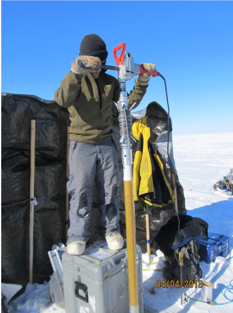
Side winder mechanical drill ( for cold firn)
