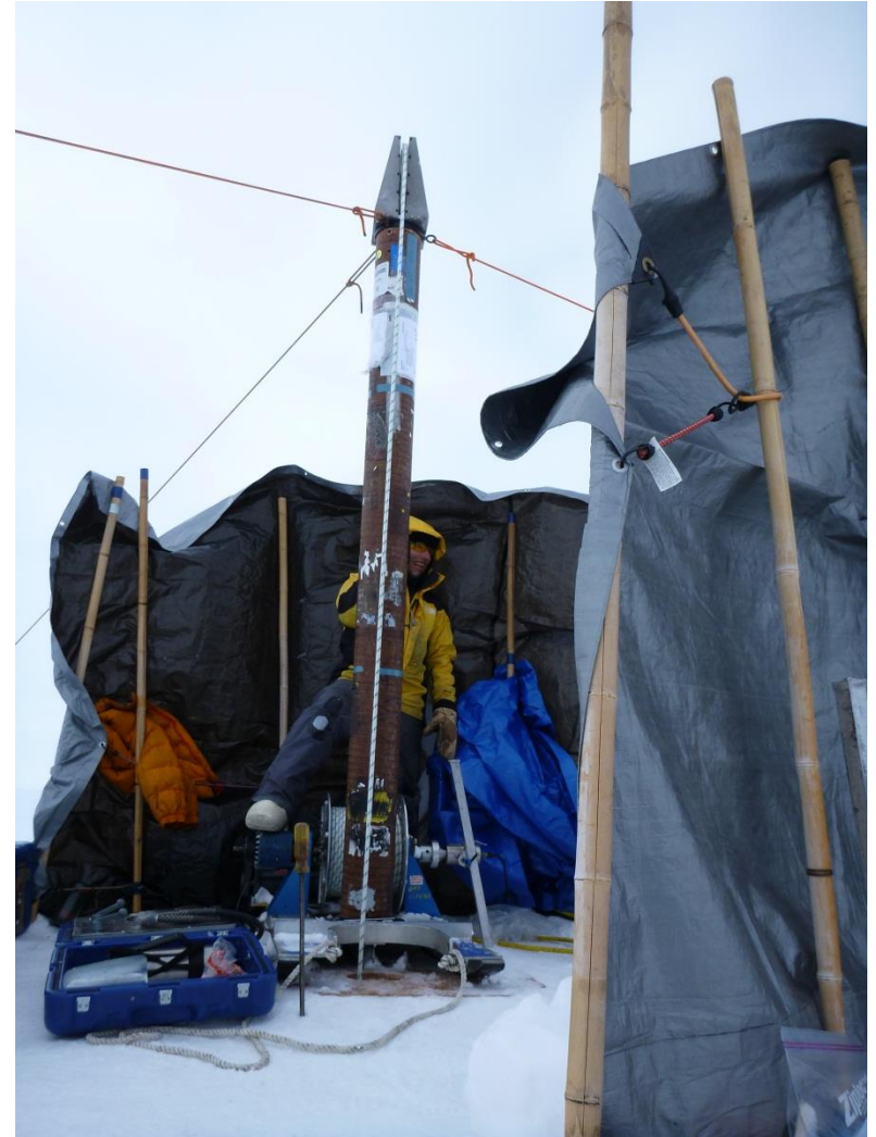
Electrothermal drill (for wet firn & 0C ice)
