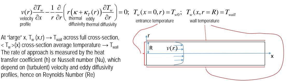
Proper formulation of multi-dimensional heat transport boundary value problem for transfer of internally dissipated mechanical energy (converted to thermal energy) from fluid to conduit walls
