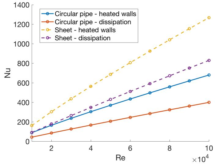
Nu for dissipated energy transfer is smaller than for transfer from heated walls even in sheet geometry
