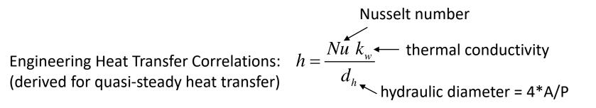
Clarke (2003) used the classical Dittus-Boelter correlation – based on heat transfer from heated walls (perimeter) of a duct to the bulk fluid, also applicable for warmer fluid and cooler walls – neglect thermal energy resulting from mechanical energy dissipation
