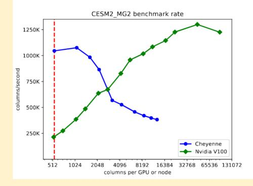
This figure shows the number of subcolumns that can be handled per second by MG2 vs a GPUized version of MG2. Courtesy of John Dennis.
