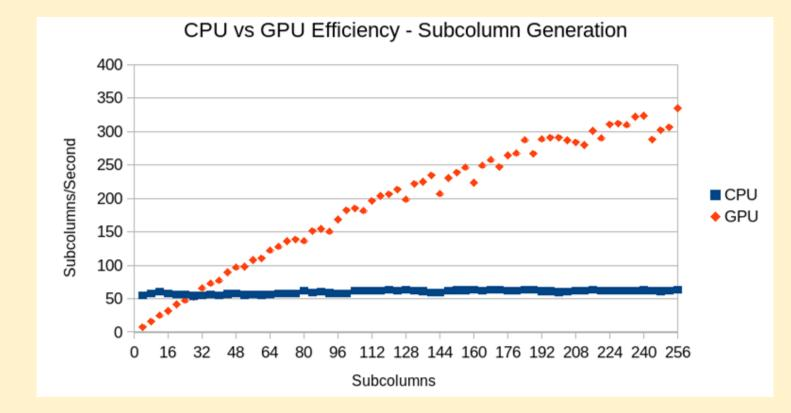
This figure shows the number of subcolumns that can be generated per second using a single Intel Xeon CPU core, compared to using a P4000 GPU. The test was run with a single column model.
