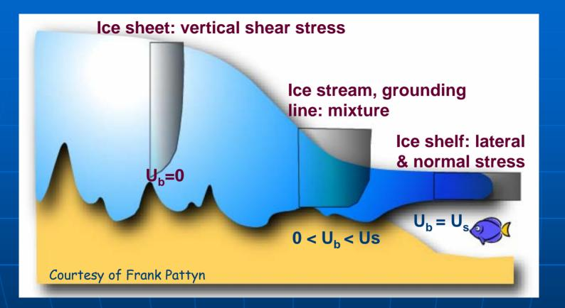
Current ice sheet models are fairly reliable for slow-moving ice sheet interiors, but not for fast-moving ice streams and outlet glaciers.
