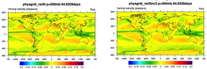
When using a 3x3 physics grid, cell averaged quantities reduce extrema seen by the physics. Vertical pressure velocity is less noisy near steep topography (Andes, Himalayas)
