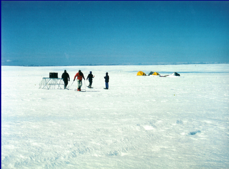
MICROTOP'97-'99: Measurement of Ice Surface Roughness with the Glacier Roughness Sensor (GRS) in the Jakobshavn Isbræ Drainage Basin:
