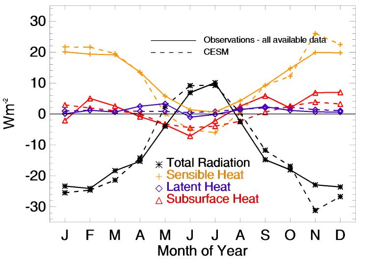
Subsurface Heat = C + S Heat Storage in the upper layer of snow plus conductive flux below this layer.
