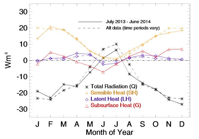
G = C + S Heat Storage in the upper layer of snow plus conductive flux below this layer.
